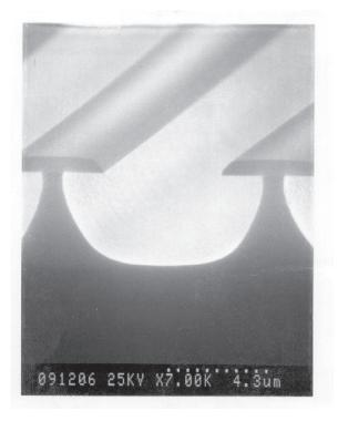
**Figure 3.** SEM of a trench etched in silicon in a  $SF_6$  plasma, showing large undercut beneath the mask.
