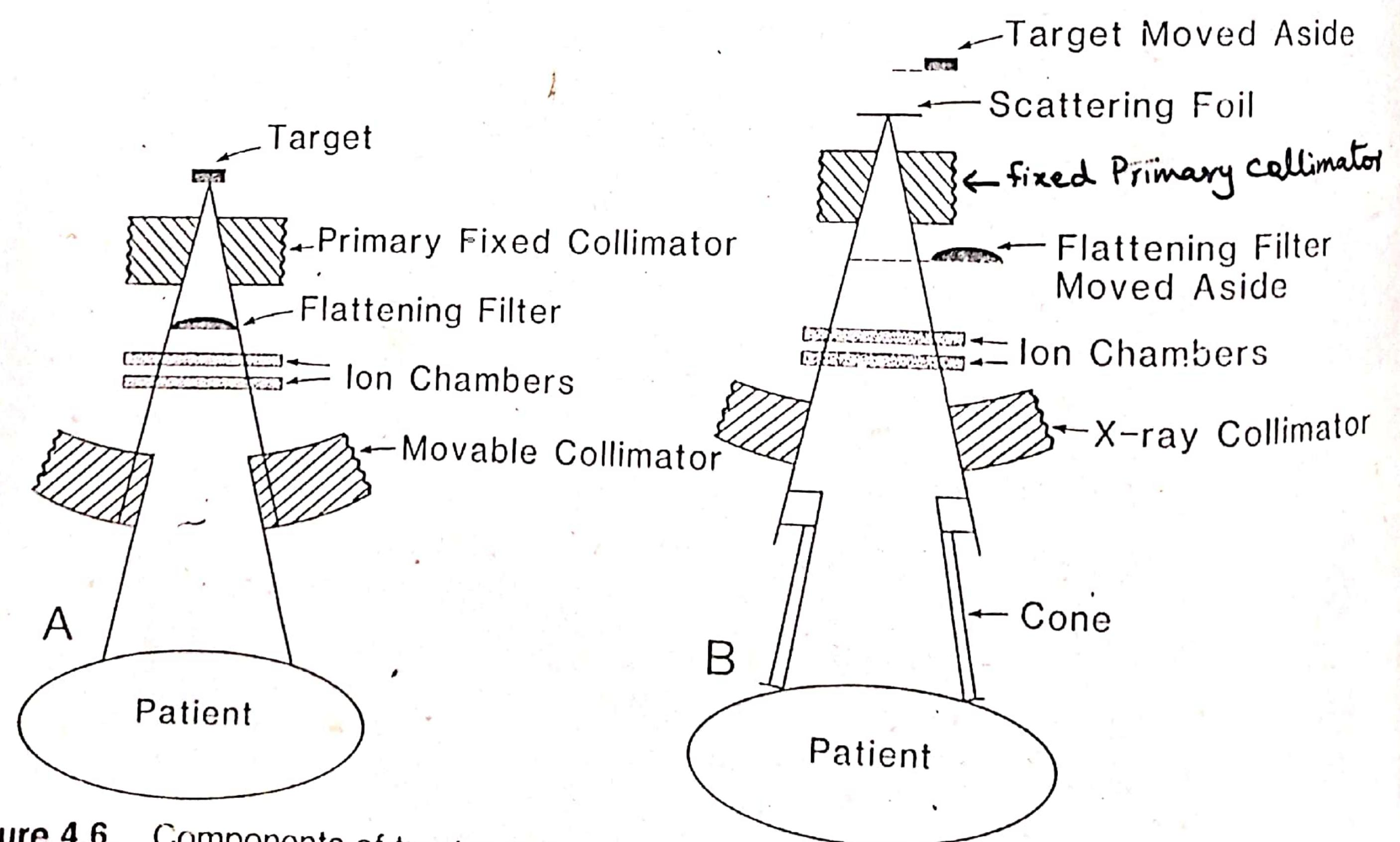
Figure 4.6. Components of treatment head. (A) X-ray therapy mode; (B) electron therapy mode
