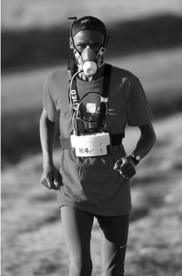
FIGURE 8.3 Portable indirect calorimetry device. (Photo courtesy of Cosmed USA, Inc.)
