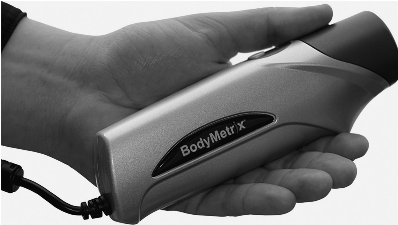
FIGURE 9.3 Ultrasound device used for the measurement of body composition.
