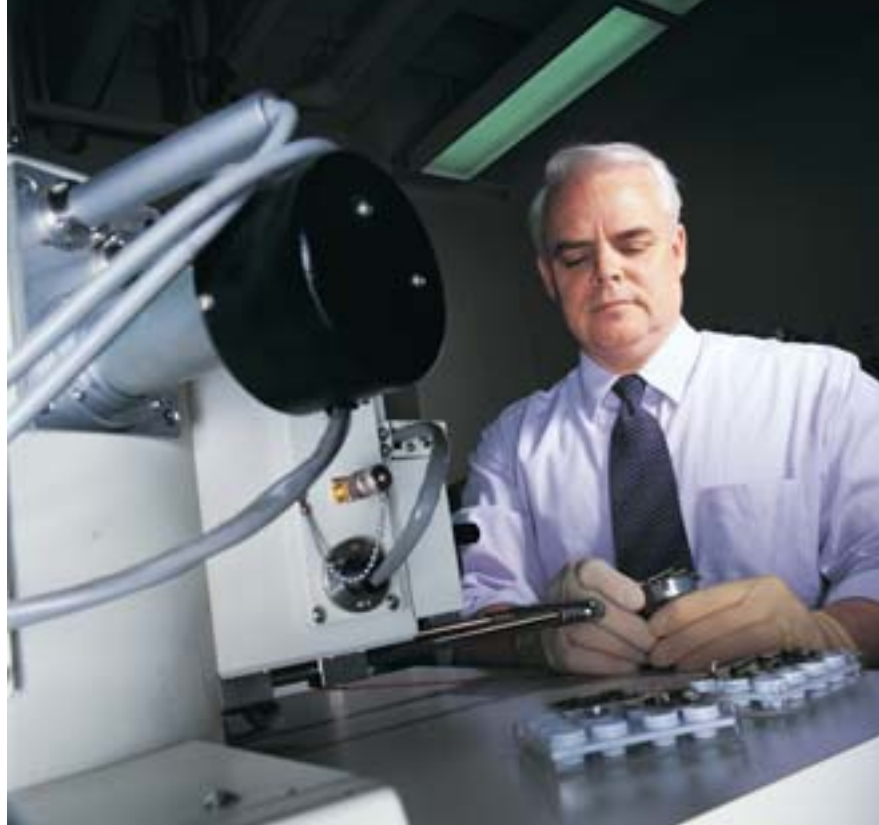
TELLTALE TOOL MARKS become visible when the author examines ancient Indus Valley artifacts with a scanning electron microscope at the University of Wisconsin–Madison.
