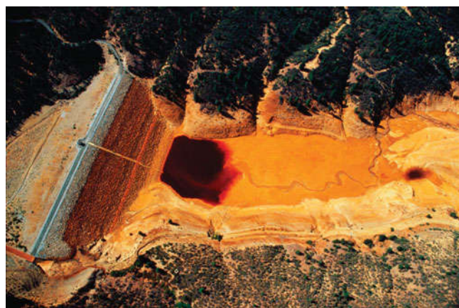
FIGURE 19.8 Aerial view of an acid mine drainage holding pond adjacent to an iron mine (located in the mountains of southwestern Colorado).
