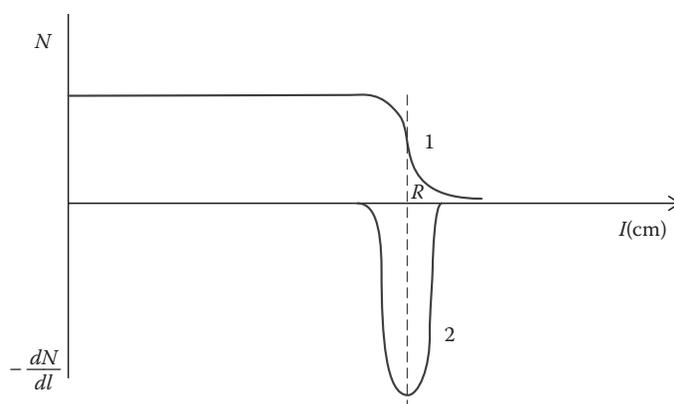
**FIGURE 1.2** Dependence of the number of  $\alpha$ -particles on the distance from the source.  $N$  is the number of  $\alpha$ -particles on the distance  $l$ ;  $-dN/dl$  is the number of  $\alpha$ -particles with the path  $l$ ;  $R$  is the medium path of  $\alpha$ -particles.
