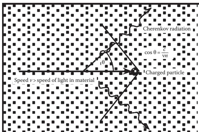
**FIGURE 1.4** The speed  $v$  of the charged particle is greater than the speed  $c/n$  of light in the material;  $n$  is the refractive index.
