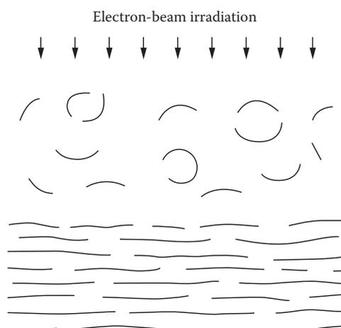
**FIGURE 1.10** Formation of fullerene-like shells above the graphite surface under electron-beam irradiation.
