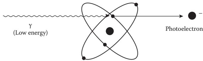
FIGURE 1.5 Photoelectric effect.
