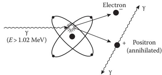
FIGURE 1.7 Electron–positron pair production.
