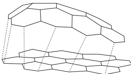
**FIGURE 1.11** Zipper variant of the coagulation mechanism of formation of fullerenes from two aromatic fragments.
