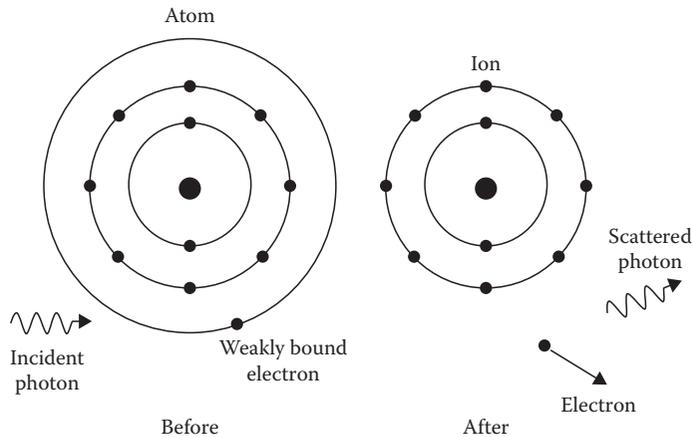
FIGURE 1.6 Compton scattering by a weakly bound electron.
