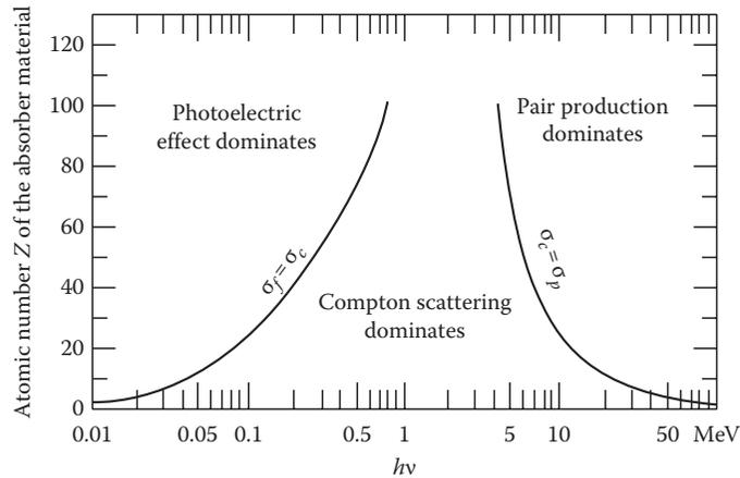
FIGURE 1.9 The relative importance of various processes of  $\gamma$ -radiation interaction with matter.
