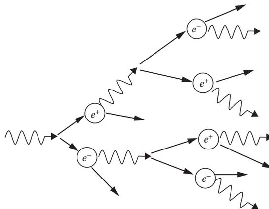
FIGURE 1.8 An electron–photon cascade.
