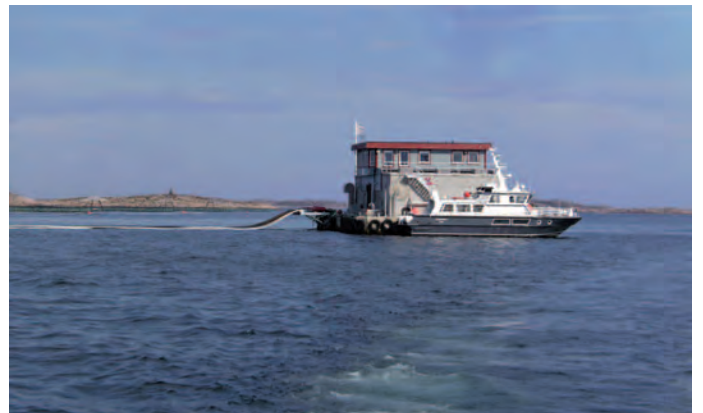
ABOVE, FIGURE 6. TOP: Offshore salmon farm producing 12,000 ton/yr in Norway. BOTTOM LEFT: Pneumatic feed distribution system. BOTTOM RIGHT: Floating 4-store building for feed storage and control room.
