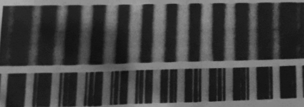
FIGURE 43-1. The diffraction pattern for a grating with (a) two slits and (b) five slits. Note that, in the case of the five-slit grating, the fringes are sharper (narrower), and secondary maxima of low intensity appear between the bright principal maxima.
