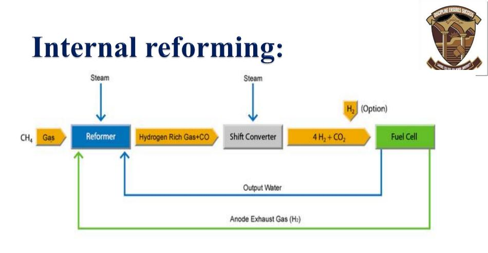
Reformer Reaction  $CH_4 + H_2O \rightarrow CO + 3H_2$  $\triangle H = +205,8 \text{ kJ/mol}$
