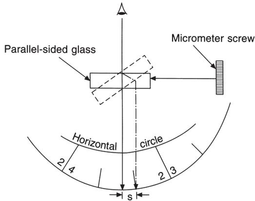
**Fig. 5.5** *Micrometer*
