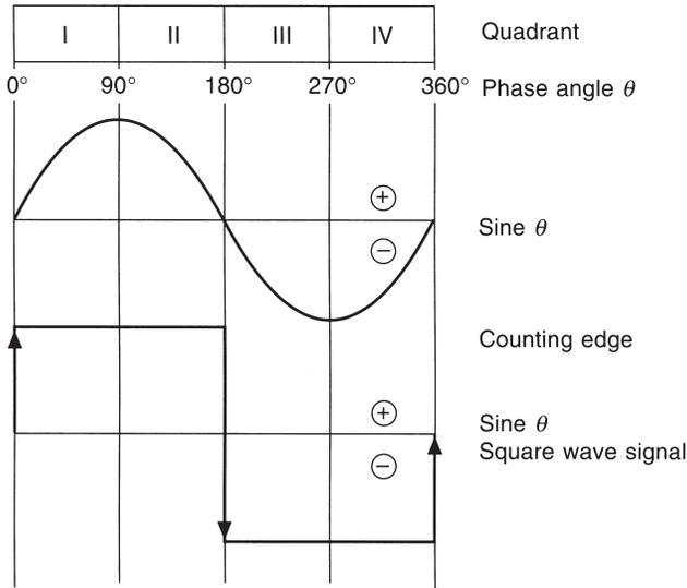
**Fig. 5.10** *Sine wave to square wave modulation*
