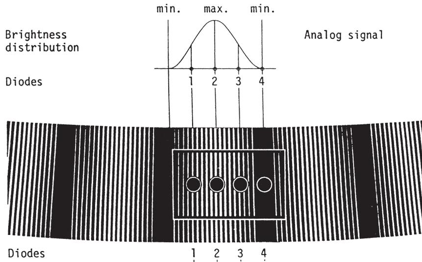
**Fig. 5.11** Fine reading using moiré pattern brightness
