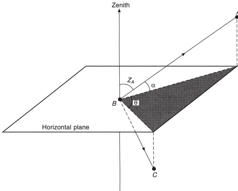
Fig. 5.1 Horizontal, vertical and zenith angles
