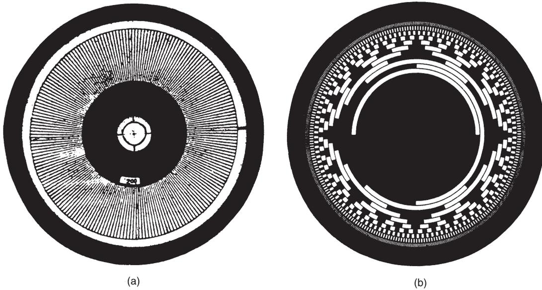
**Fig. 5.9** (a) *Incremental disk*, (b) *binary coded disk*
