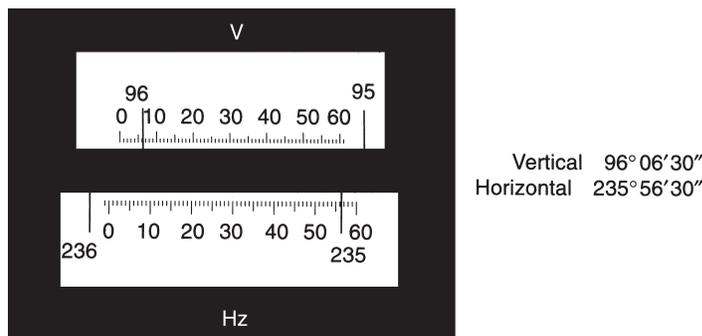
Fig. 5.4 Wild T16 direct reading theodolite
