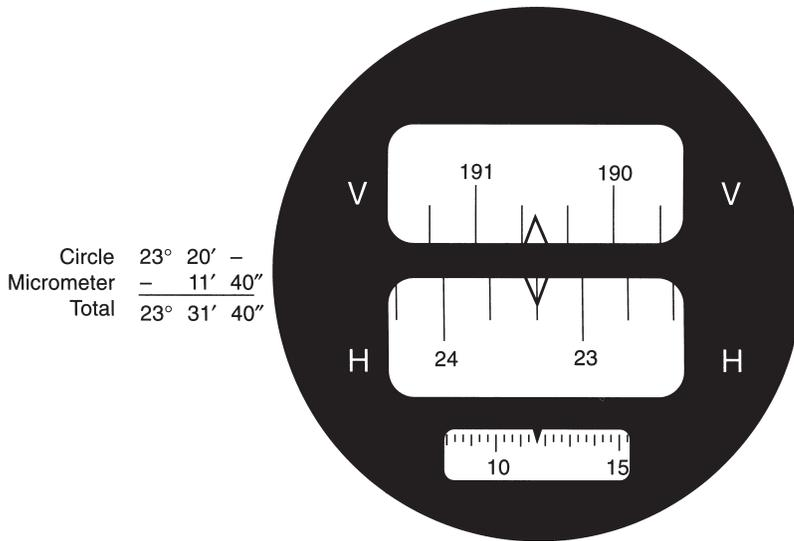
**Fig. 5.6** *Watts Microptic No 1 theodolite reading system*
