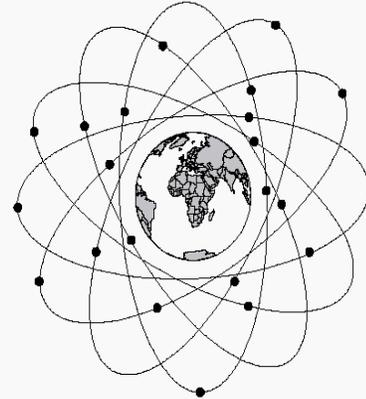
The satellites continuously orient themselves to ensure that their solar panels stay pointed towards the sun, and their antennas point toward the earth. Each satellite carries 4 atomic clocks.
